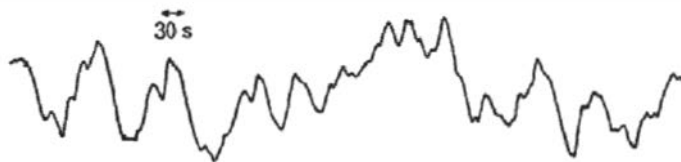
Fig. 1.1. Brownian motion caused by incessant impacts of gas molecules against a mirror suspended in a dilute gas [1.5]
